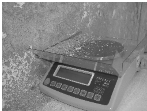
Fig. 11: Balance for the collection of debris falling from the wall
