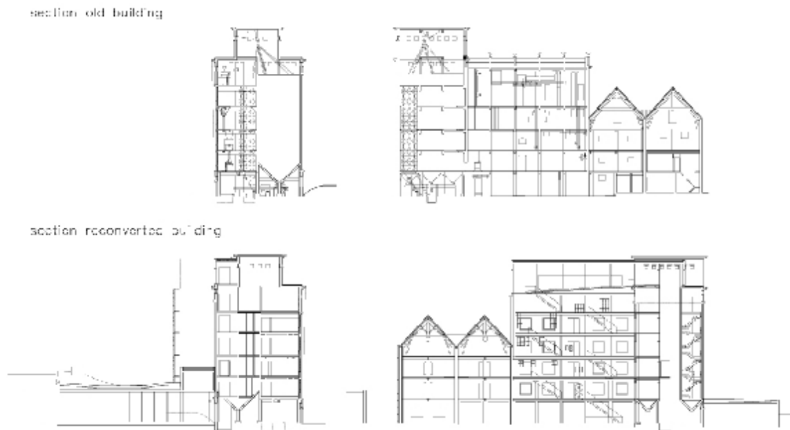
Fig. 3: Section of the old and reconverted building
